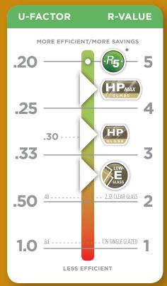
The lower the U-Factor, the greater the insulation value. R-Value is the inverse (R=1/U) of the U-Factor. Total Unit Factors determined per NFRC-100 (National Fenestration Rating Council). Chart shows relationship between performance and Ply Gem Windows glass package options, not including energy package upgrade.
